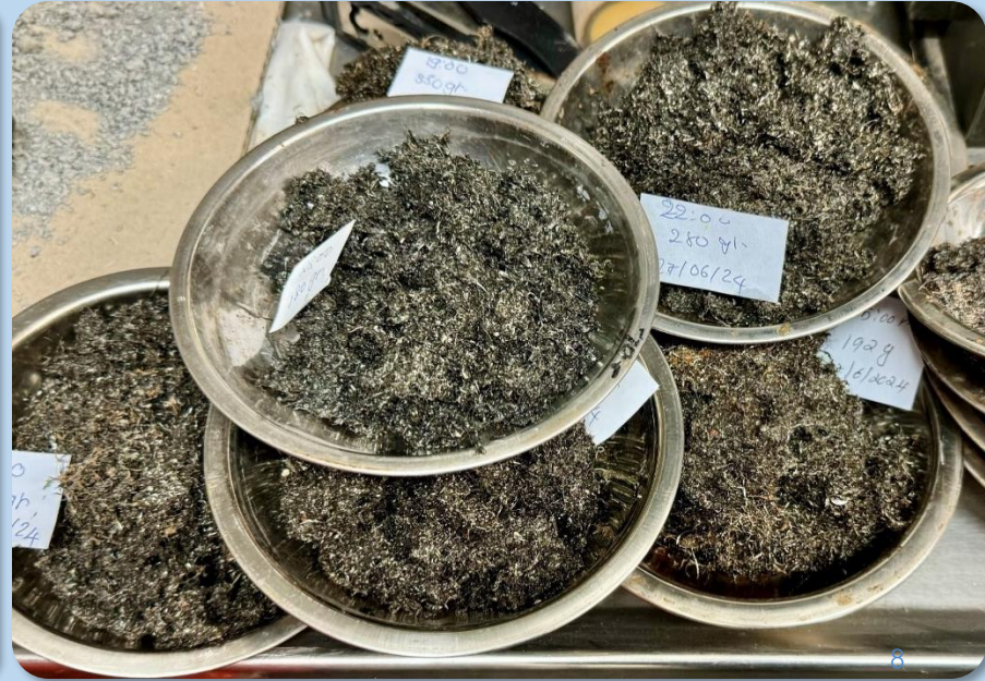
After milling a window in the target casing
