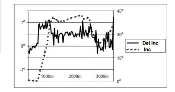
A 15 station IDT was run to find out if these inclination differences are acceptable relative to the tool error models assigned to the surveys. The MWD survey was assigned to the SPE-WPTS sag corrected MWD error model, and the gyro survey to the stationary error model recommended by the gyro service provider. The following test result was achieved:
