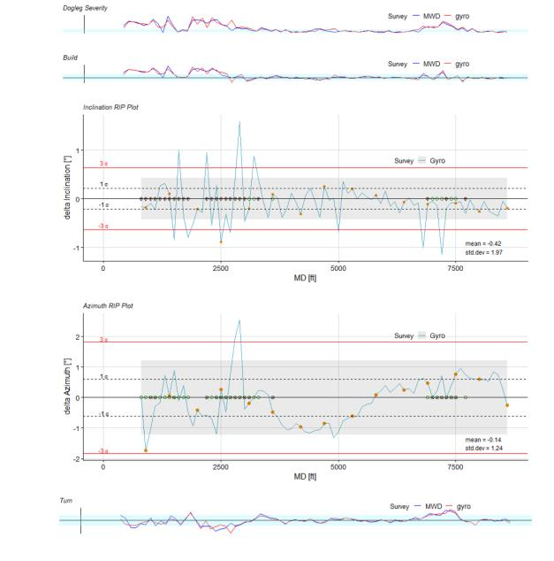
Shaded areas: grey = 2 sigma tolerance level light blue = dogleg severity: between 0 and 1, turn and build: between -1.5 and 1.5 Well Stations: orange point = Chi-Square test, green circle = high dogleg severity, red cross = high build, pink X = high turn
