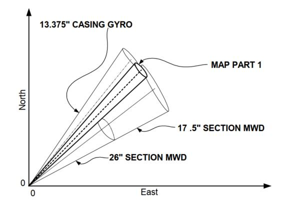
Fig. 4 - Schematic for the same planned directional well, for the first series of drilling surveys and the first casing gyro survey, where the MAP technique is used to obtain a more accurate updated wellpath position, from which drilling progress will continue.
