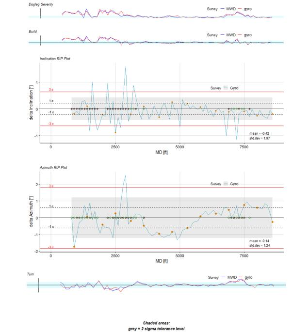
light blue = dogleg severity: between 0 and 1, turn and build: between -1.5 and 1.5 Well Stations: orange point = Chi-Square test, green circle = high dogleg severity, red cross = high build, pink X = high turn
