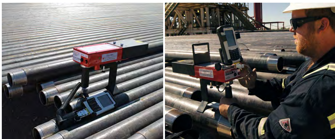
Figure 68: Drill pipe length measurement using laser (image courtesy of Digi-Tally)
