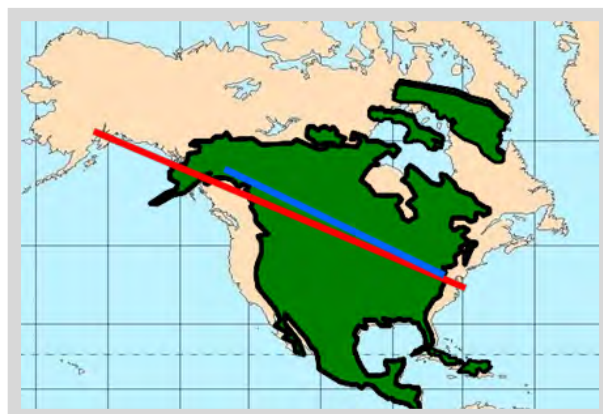
Figure 20: The plane surface can be tangent or secant to the ellipsoid. Secant even the distortion.
