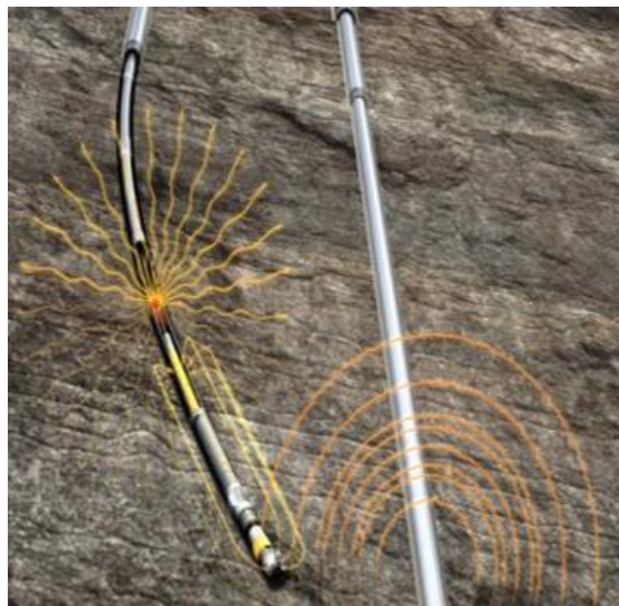
Figure 15—AI-AMR system diagram. No target well access. A wireline conveyed AMR tool injects the formation with AC current creating an induced magnetic field in the target well casing.
