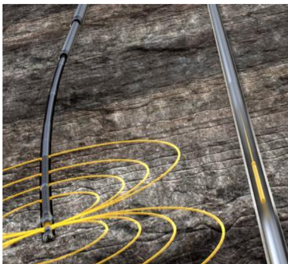
Figure 11—Typical rotating magnet AMR system diagram showing the rotating magnet sub near the bit and the wireline conveyed directional sensor in the target well.
