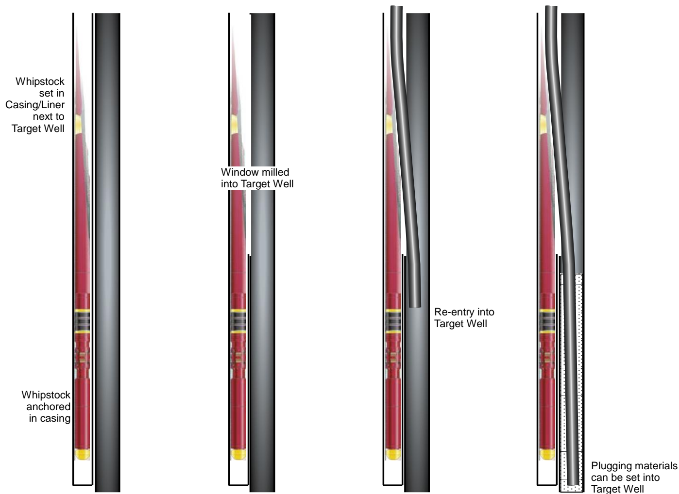
Figure 89—Cased hole whipstock milling method concept
