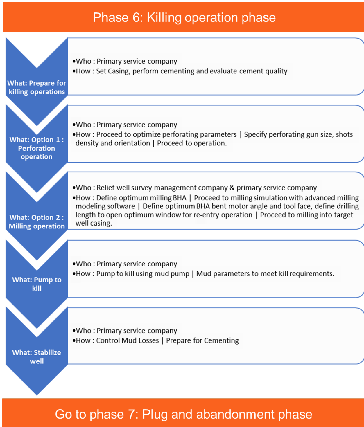
Figure 90—Phase 6: Killing operation phase key tasks and responsibilities
