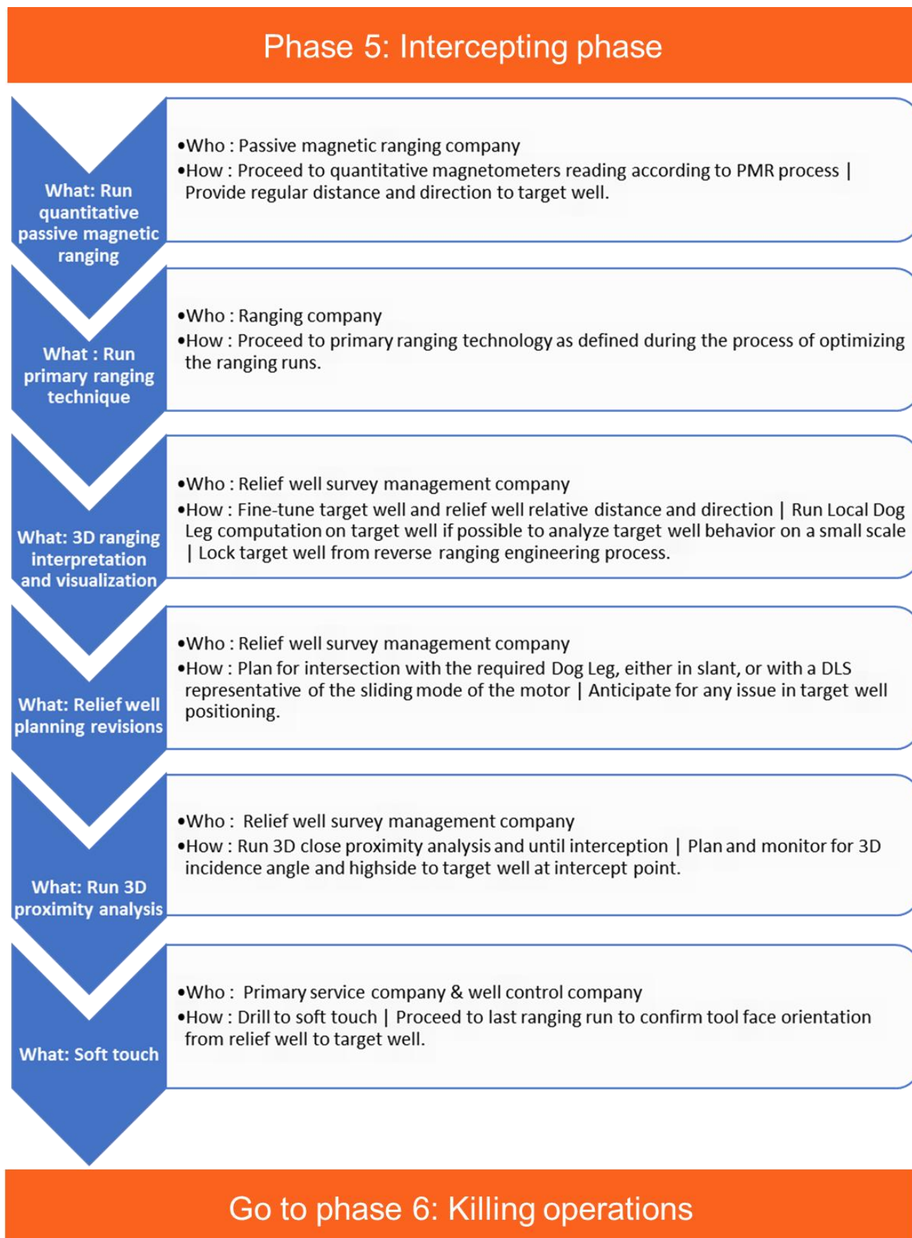
Figure 79—Phase 5: Intercepting phase key tasks and responsibilities.
