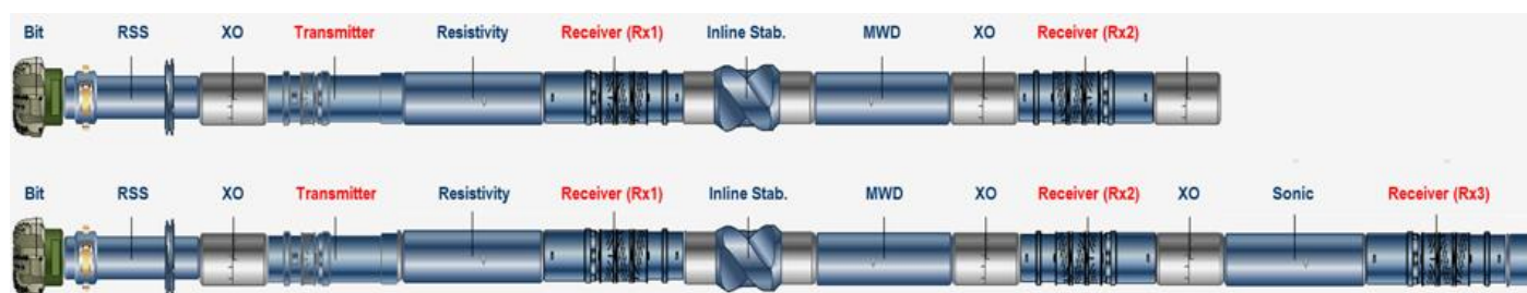
Figure 40—The location of the resistivity transmitter and receivers in the two different example BHAs
