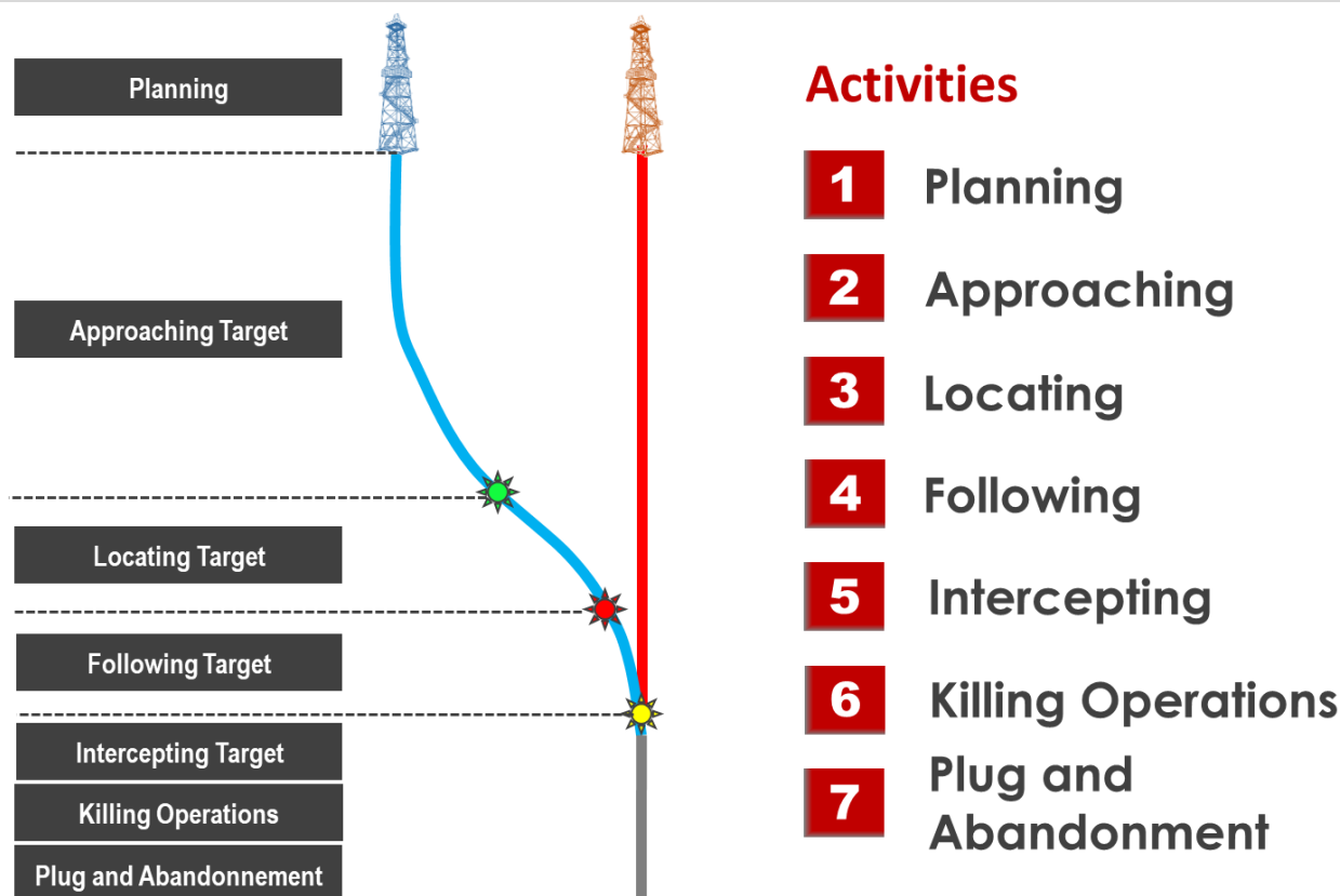
Figure 50—The core of the relief well process is the workflow, consisting of seven phases
