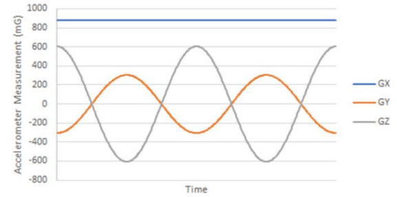
Example Accelerometer Data During Rotation
