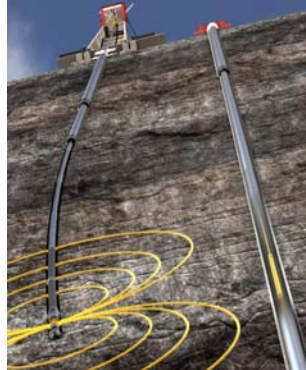
Access Dependent Active Magnetic Ranging
