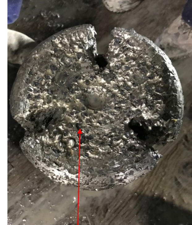
Mill face showing 2-3/8" tubing wear pattern
