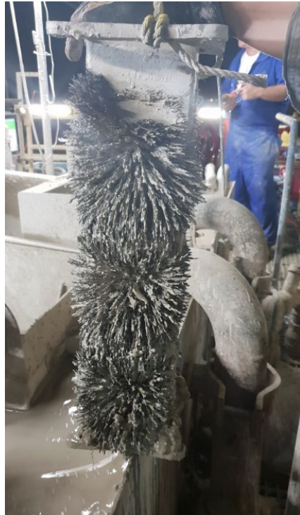
Milling cuttings from ditch magnet
