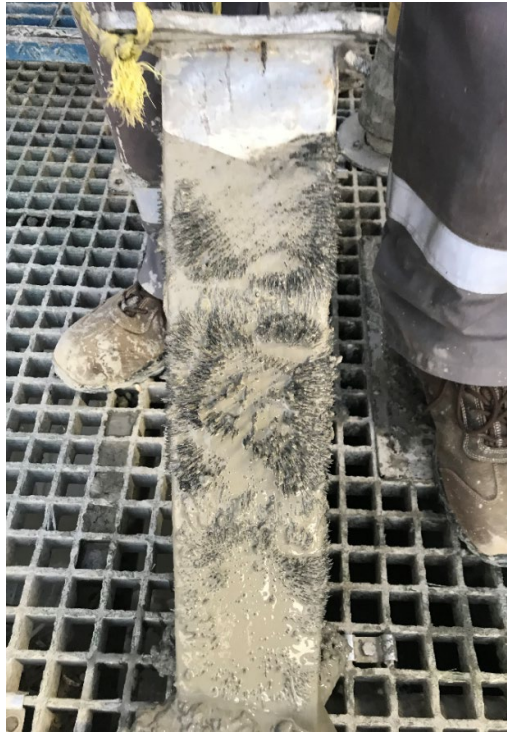
Milling cuttings from ditch magnet
